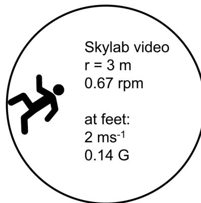
Fig. 4. Running on Skylab. By analysis of Skylab NASA Public Affairs Office motion film, the crewmember was running on the wall (3 m radius) at 9 seconds a revolution (0.67 rpm). At this rotation speed, the centrifugal acceleration at feet was ca. 0.14 Gz. Starting the run was difficult, since before they gained velocity, there was no mechanism to stabilize their body in microgravity. As the +Gz value at the heart level was very small, no cardiovascular effect was expected.
