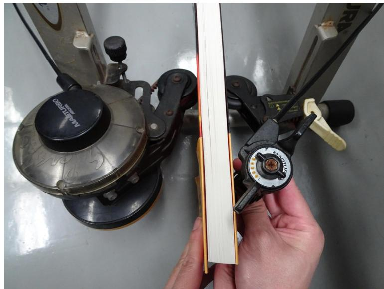
Fig. 7. An example of permanent magnet bicycle rim loader [V]. Level of load is adjustable with the dial in hand. These items are sold commercially for serious athlete riders. Its durability is excellent. The location of bicycle aluminum wheel rim is shown by a book. Rubber rollers are replaced regularly.
