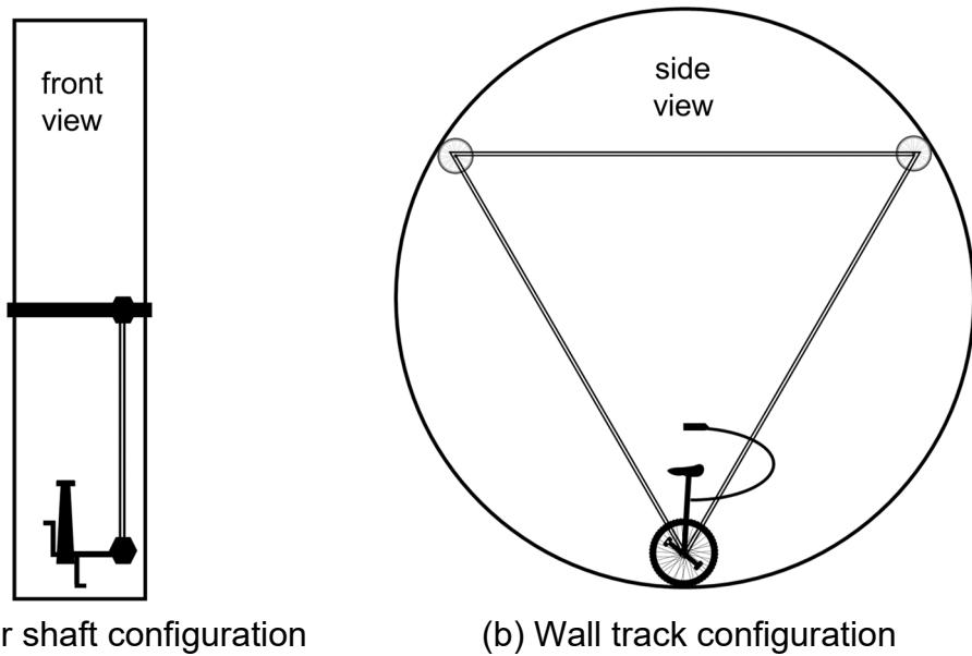
Fig. 5. Design options for an ISS human short-arm centrifuge [27], (a) front view of a swing rotating around a center shaft design. Heavy members sustain the center shaft. If motorized, this may be easier to build, (b) side view of a monicycle running on a rail on the wall. Authors' preference. Weight distribution is for the rail and the truss (triangular for this design sample). Very similar to riding a bicycle, braking is easy, inherently safe.
