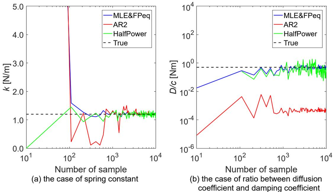
Fig. 1. Benchmark test results in terms of sample number dependency.
