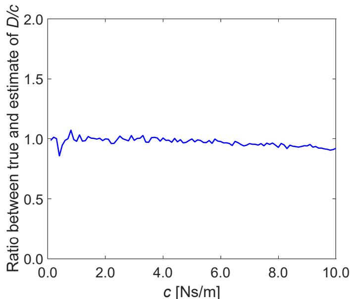
Fig. 5. Damping coefficient dependency on estimation accuracy in case of ratio between diffusion coefficient and damping coefficient.
