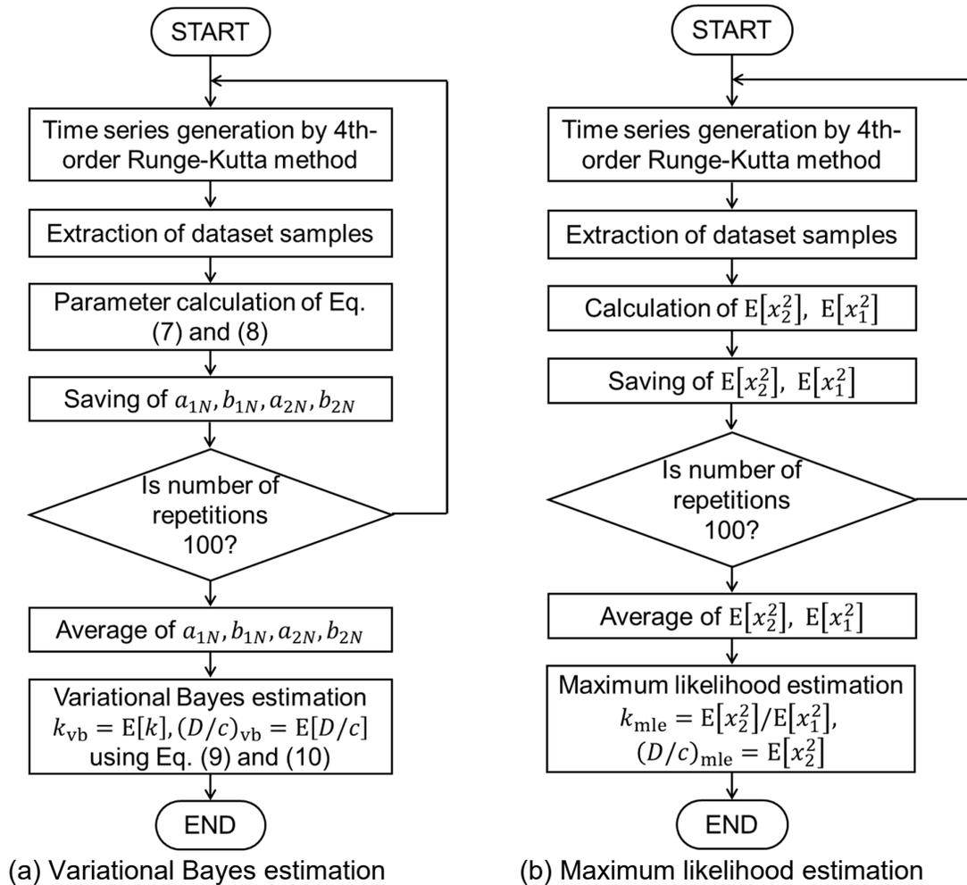
Fig. 3. Flowcharts for the numerical identification algorithm using (a) Variational Bayes estimation and (b) Maximum likelihood estimation for high-accuracy implementation.
