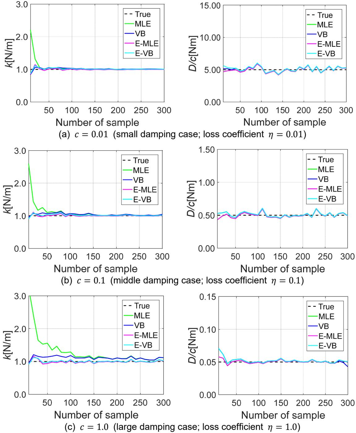
Fig. 4. Benchmark test results for the high-accuracy implementation trial. The left column shows the results for the spring constant ( $k$ ) and the right column shows the results for the ratio diffusion coefficient ( $D$ ) and the damping constant ( $c$ ). The damping constant ( $c$ ) is set to (a)  $c = 0.01$ , (b)  $c = 0.1$ , and (c)  $c = 1.0$ .
