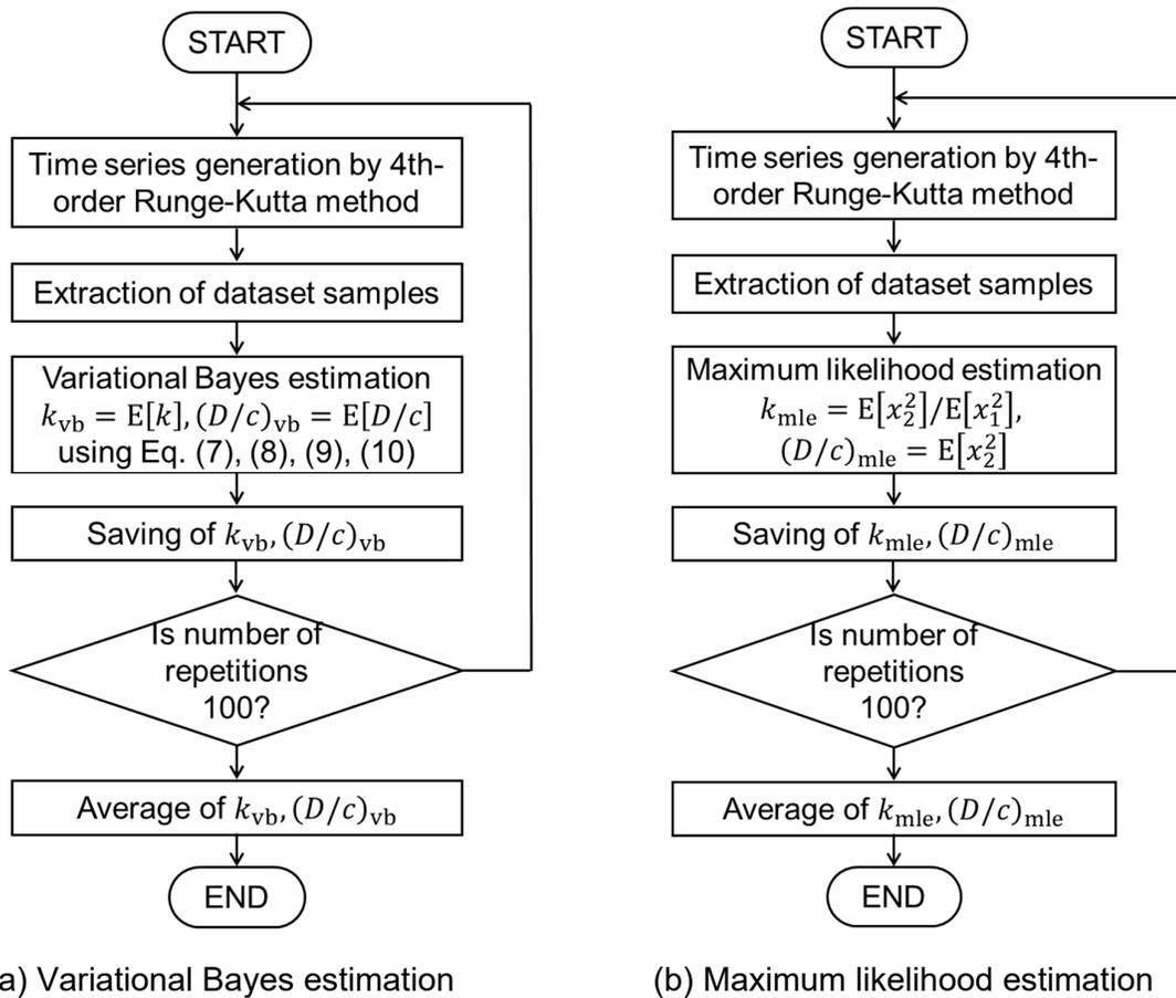
Fig. 1. Flowcharts for the numerical identification algorithm using (a) Variational Bayes estimation and (b) Maximum likelihood estimation.
