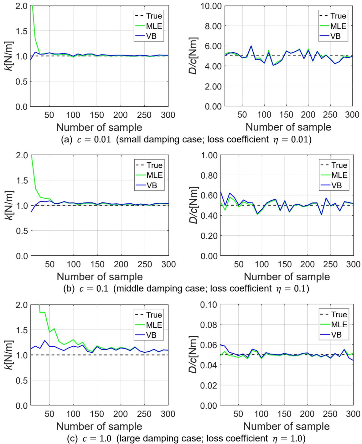
Fig. 2. Benchmark test results in terms of sample number dependence. The left column shows the results for the spring constant ( $k$ ) and the right column shows the results for the ratio diffusion coefficient ( $D$ ) and the damping constant ( $c$ ). The damping constant ( $c$ ) is set to (a)  $c = 0.01$ , (b)  $c = 0.1$ , (c)  $c = 1.0$ .
