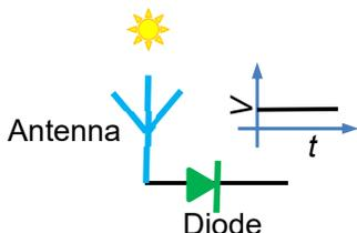
Fig. 2. Principle of the optical rectenna.
