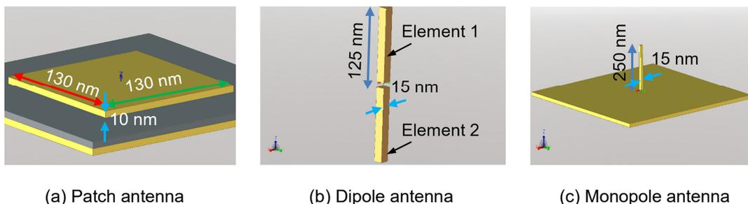
Fig. 5. Structures of antennas.
