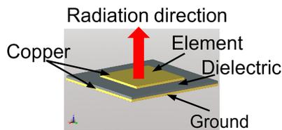
Fig. 4. An example of a square patch antenna.
