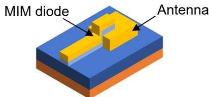
Fig. 3. Diagram of an optical rectenna.
