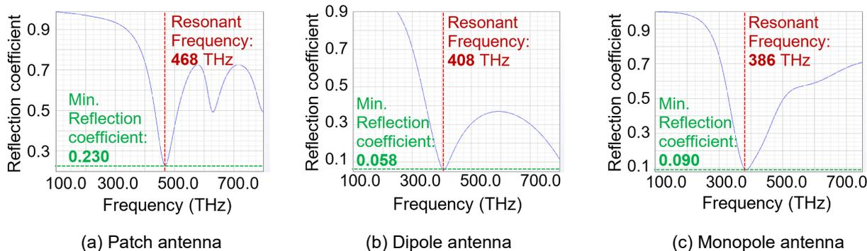
Fig. 6. Reflection coefficient as a function of frequency.
