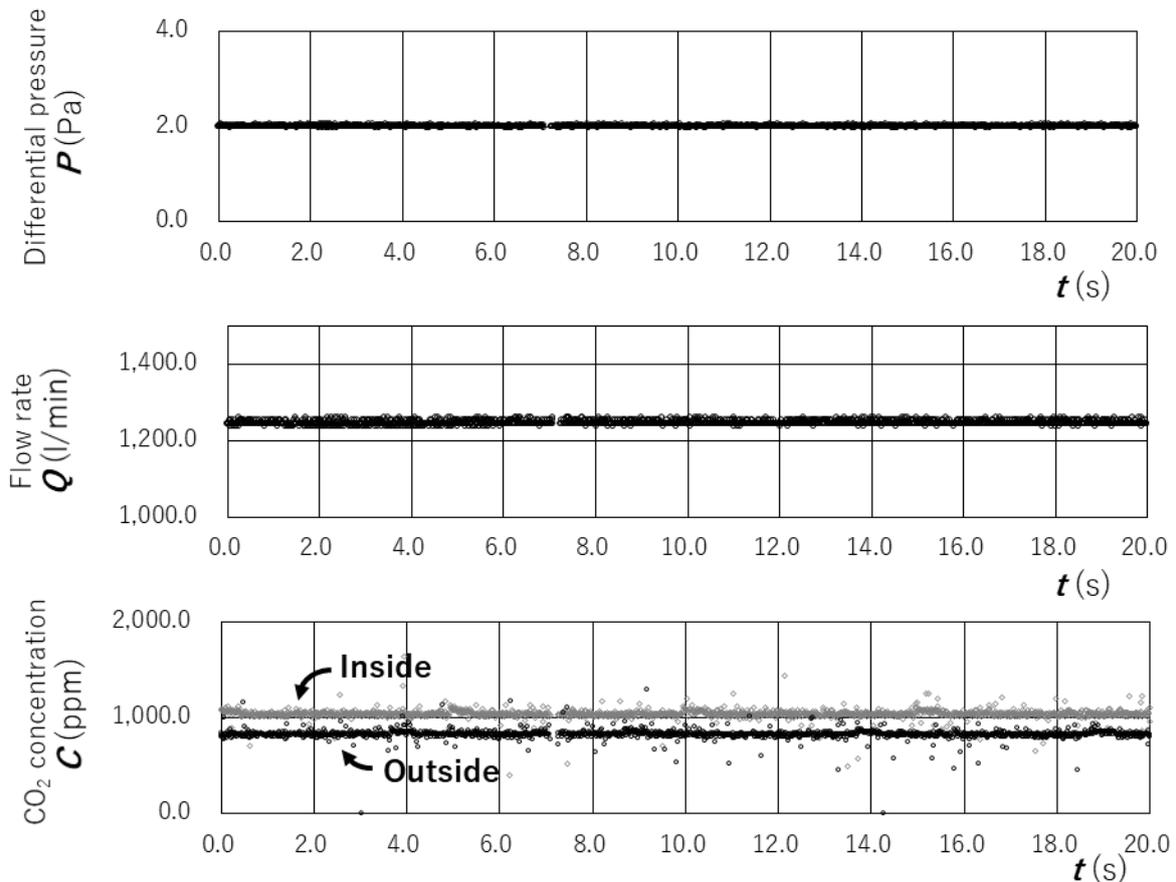
Fig. 3 Time series of control parameters during the operation
