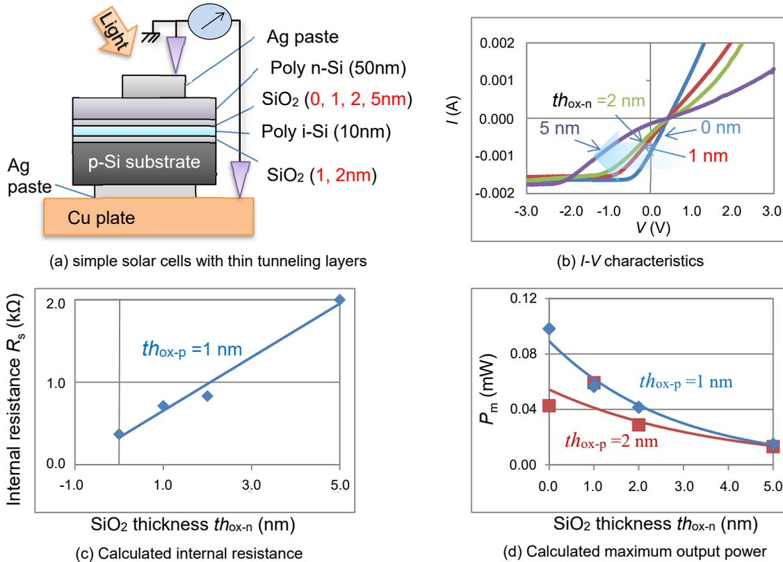
Fig. 3. (a) Schematic of simple solar cells with thin tunneling layers. (b)  $I$ - $V$  characteristics of solar cells with a thickness  $th_{ox-p}$  of 1 nm. (c) Calculated internal resistance as a function of  $SiO_2$  thickness  $th_{ox-n}$ . (d) Calculated maximum output power  $P_m$  as a function of  $SiO_2$
