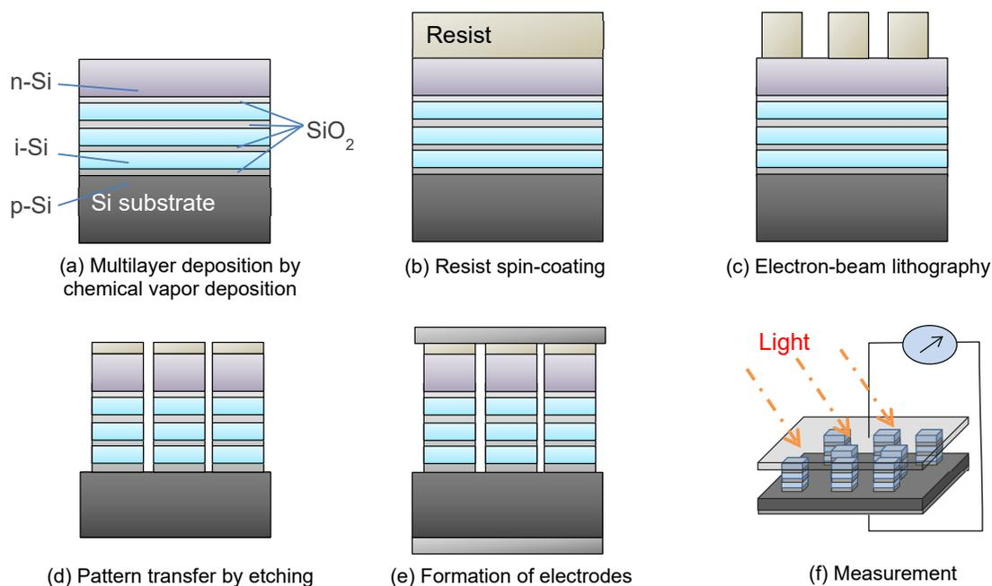
Fig. 2. Schematic of processes of fabrication and measurement of a quantum dot solar
