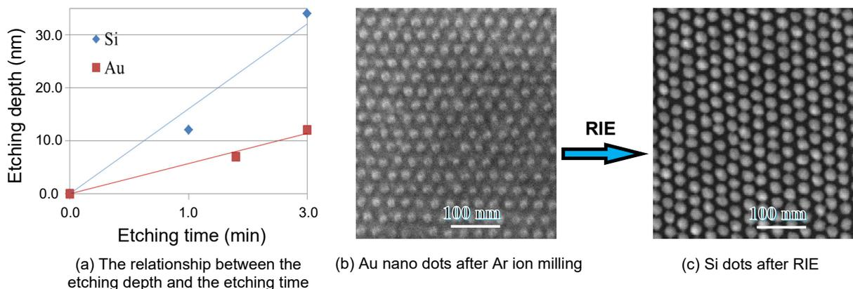
Fig. 6. The second step etching.
