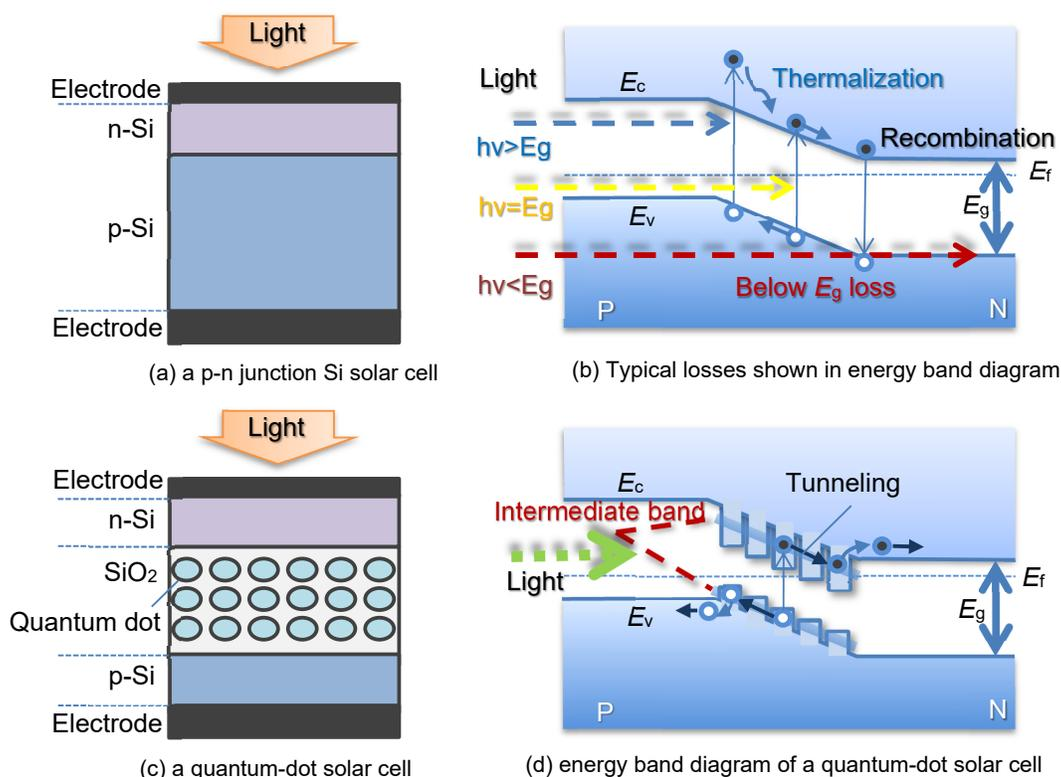
Fig. 1. (a) Schematic diagram of a p-n junction Si solar cell. (b) Typical losses shown in energy band diagram. (c) Schematic diagram of a quantum-dot solar cell. (d) Schematic of energy band diagram of a quantum-dot solar cell.
