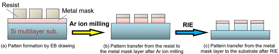
Fig. 4. Nanofabrication of quantum dots with a 2-step etching method.
