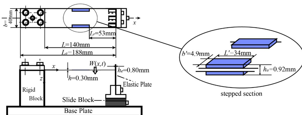
Fig. 1. Beam and fixture
