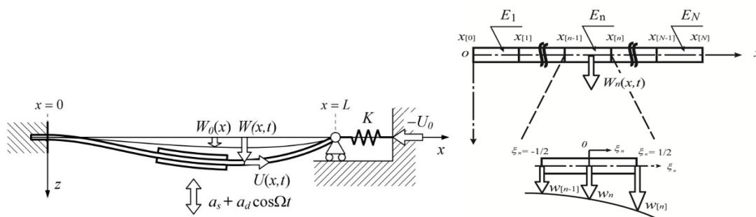
Fig. 2. Analytical model of a stepped beam
