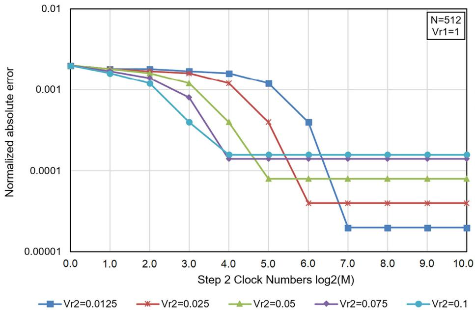
(b) With the reference voltage  $V_{r2}$ , which is 10 times smaller than that in Fig. 5 (a)
