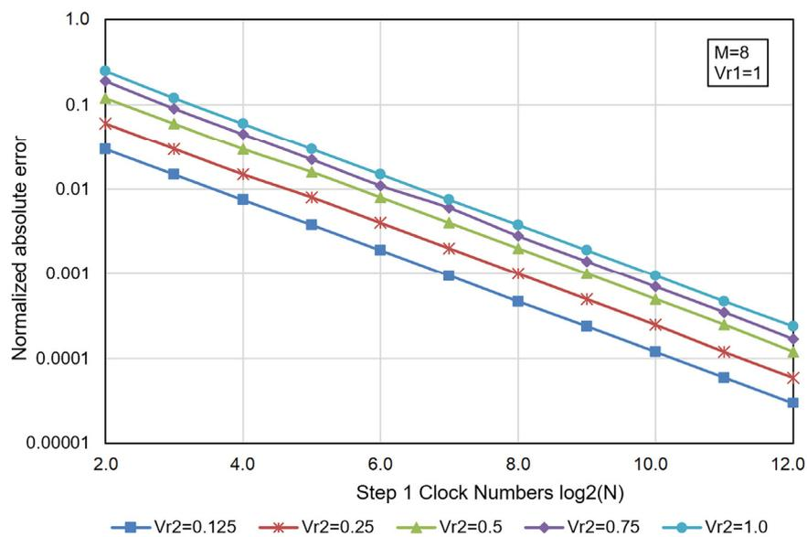
Fig. 5. Simulation results of the two-step incremental ADC as a parameter of the reference voltage Vr2 with the various number N of the step 1 clock cycles and the fixed number M (=8) of the step 2 clock cycles.
