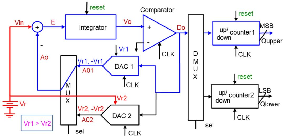
Fig. 8. Self-calibration mode:  $V_{r2}$  is measured using the incremental ADC circuit itself with the reference voltage  $V_{r1}$ .
