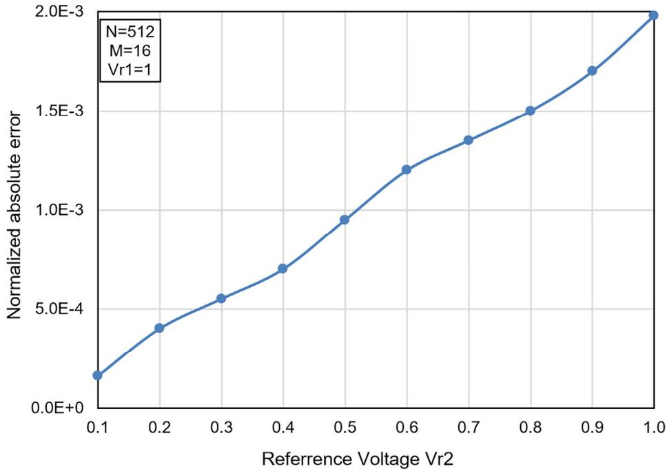
Fig. 7. Simulation results of the two-step incremental ADC operation step 2 with various reference voltage Vr2 for N=512 and M=16.
