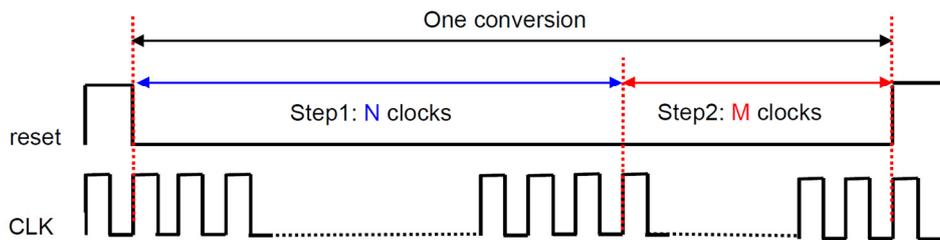
Fig. 3. Two-step incremental ADC operation timing chart.
