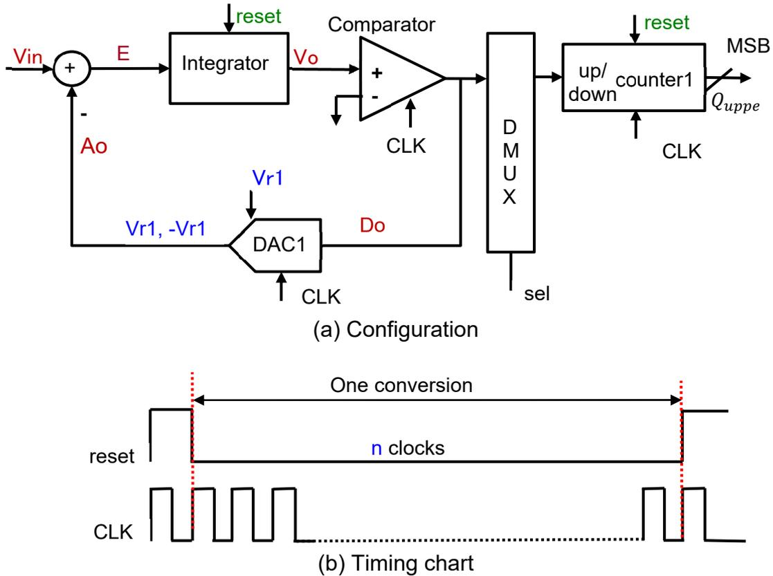
Fig.1. One-step first-order incremental ADC.
