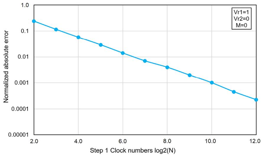
Fig. 4. Simulation results of two-step incremental ADC with only operation step 1.
