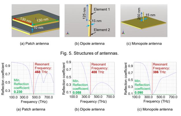
Fig. 6. Reflection coefficient as a function of frequency.
