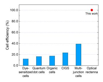
Fig. 1. Comparison of advanced technologies of solar cells and optical rectenna.
